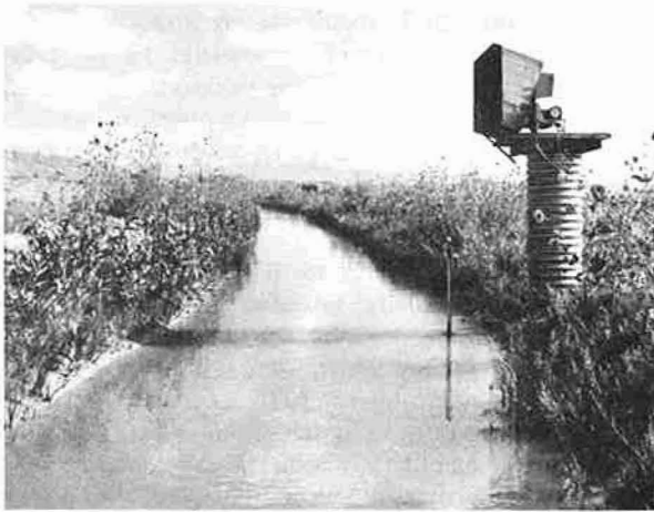
Figure 35. Showing gaging station used to determine loss in a canal. Notice also the growth of weeds along the canal.
